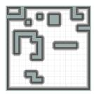
Cost maps are mathematical functions of the environment, which can be modeled using the same procedure used to create repulsive field. A grid cell of a cost map represents a movement cost, whereas in a repulsive field it represents a repulsive force value.
