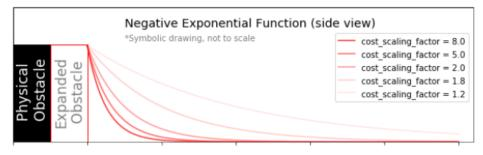
From the image below, we can observe that setting the Cost Scaling Factor higher will make the buffer zone decay faster.
